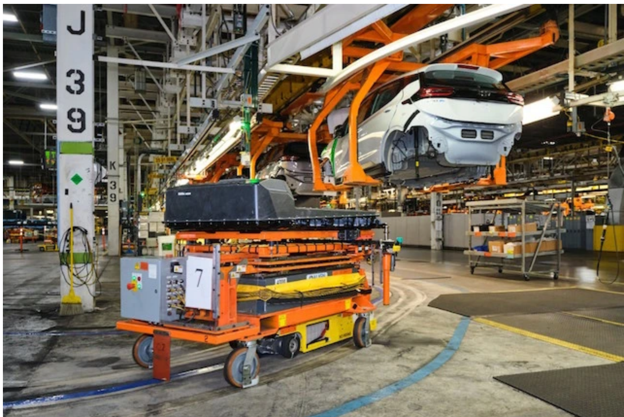
Battery packs for the 2022 Chevrolet Bolt EV go through the production line at the General Motors Orion Assembly Plant.
