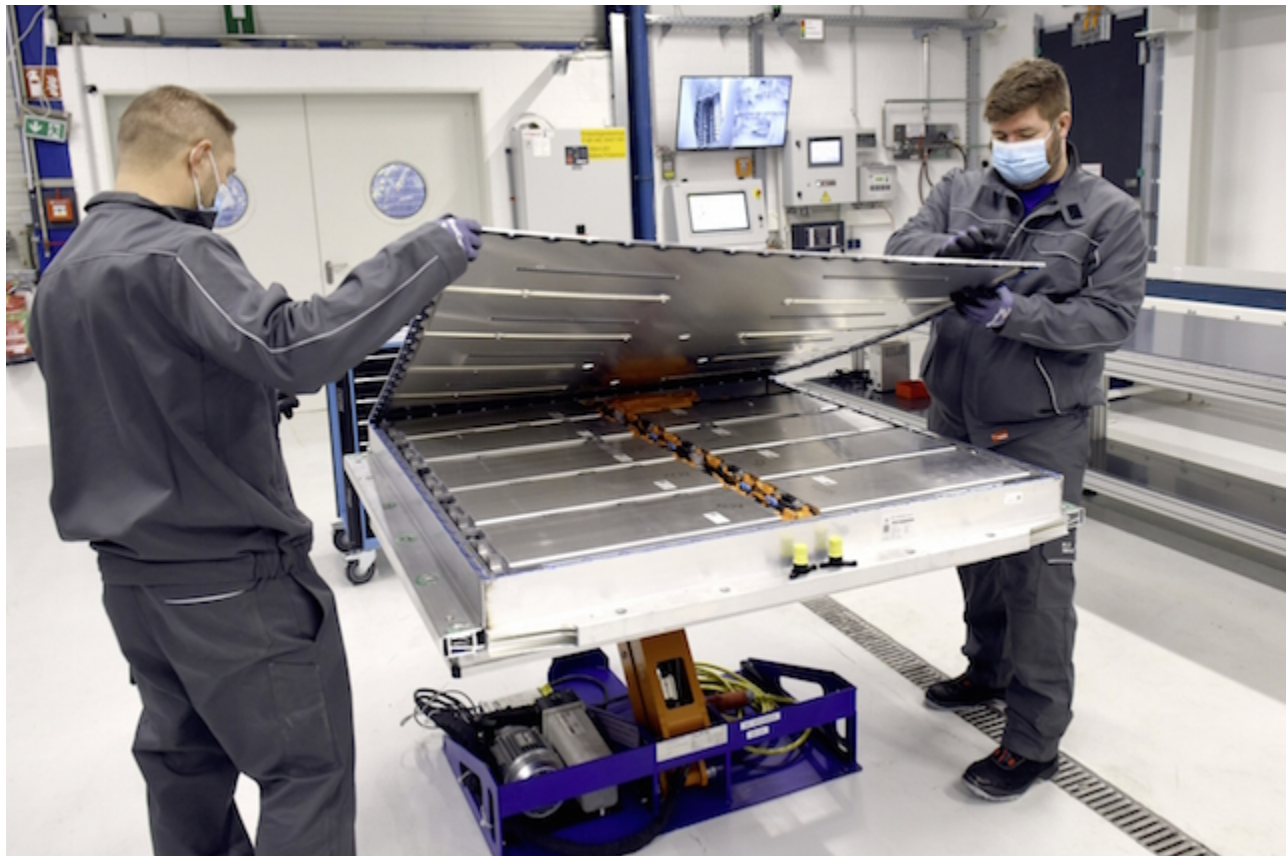
Electric battery systems are disassembled at a Volkswagen recycling pilot plant.
