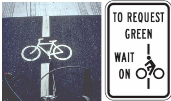
Figure 2.10. Signal activation marking and sign.
